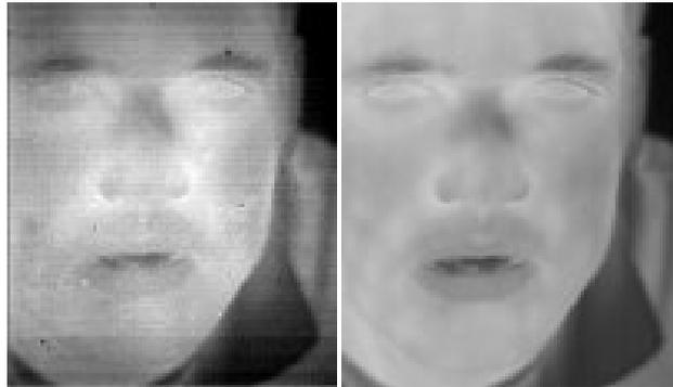
**Figure 4.** Full resolution infrared image before NUC and BPR (the left figure), and the corresponding image after the spatial NUC and BPR (the right figure).
