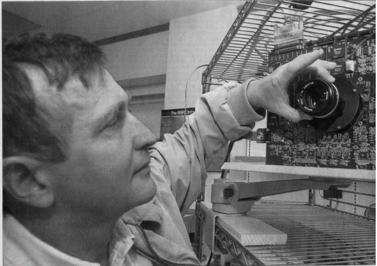
Dr. Vlad Ovod, a scientist at Nova Research in Solvang, adjusts a lens and infrared sensor that mimics the human eye and may be used in the missile defense.
